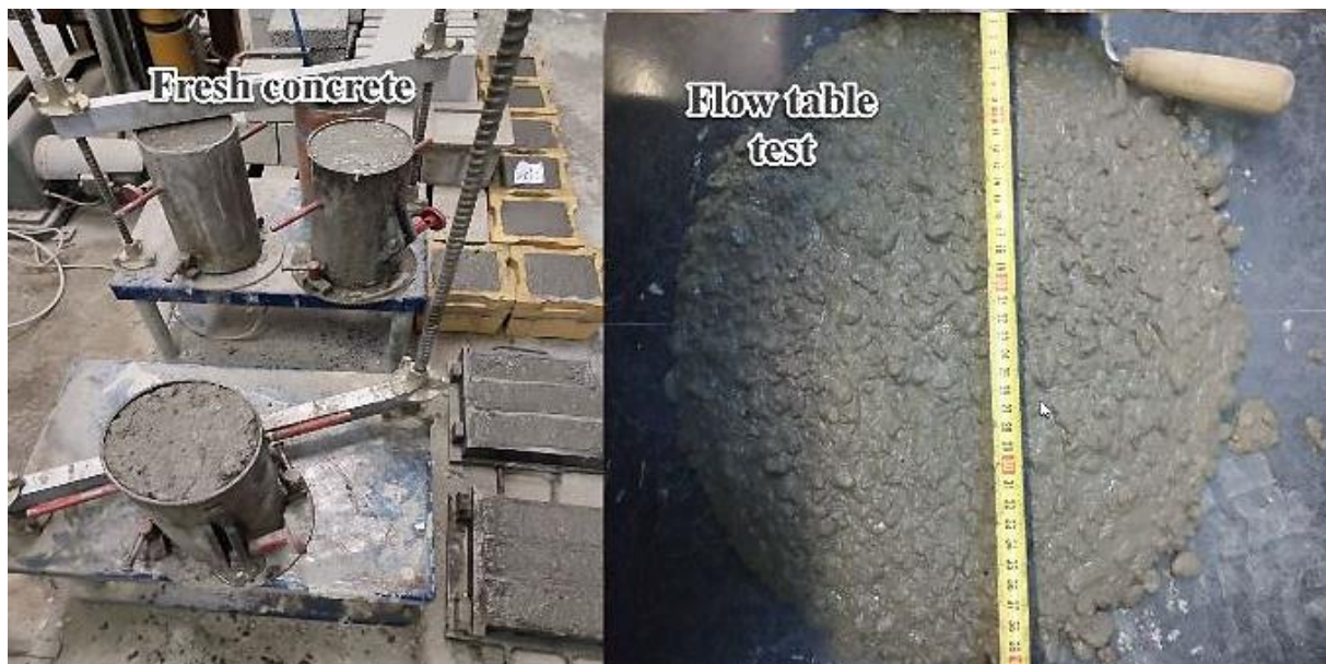
Figure 9. Flow table test of fresh concrete
