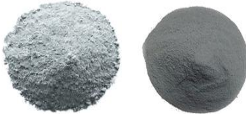
Figure 3. Fly ash (left) and silica fume (right) supplement materials [43]
